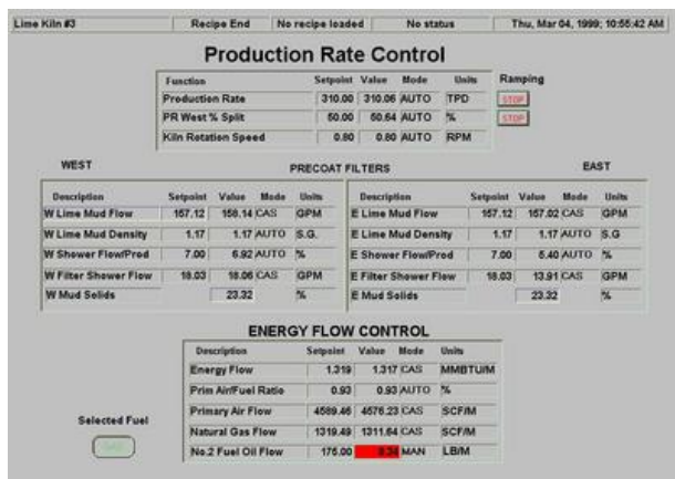
Fig. 26 Lime Kiln Production Rate Control
