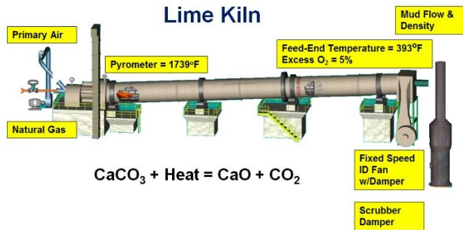
Figure 21- Lime Kiln Process
